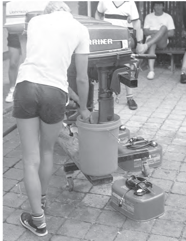
Figure 44.1 Flushing a motor in a bucket conserves water
