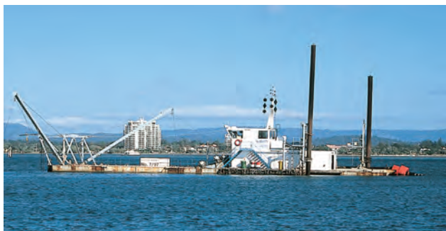
Figure 55.1 A dredge is a vessel restricted in her ability to manoeuvre (Rule 27)
