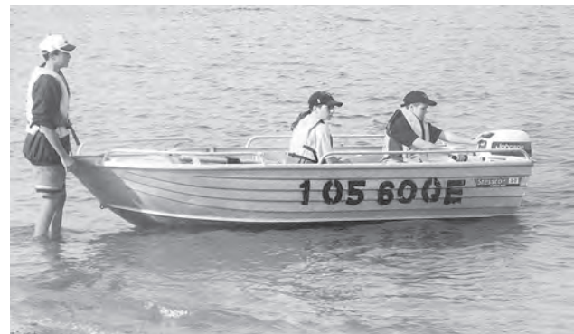
Figure 27.4 Always start the motor from inside the boat
