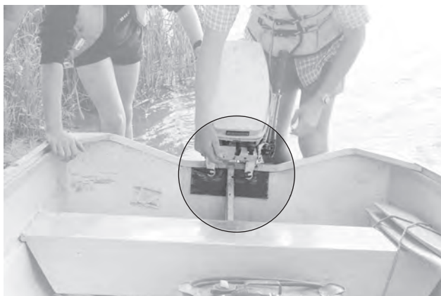
Figure 27.4 Always start the motor from inside the boat
