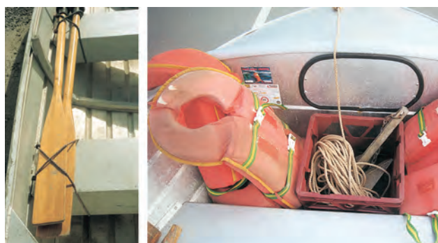
Figure 10.1 Safety items should be easy to get at and safely stowed so they do not hinder movement in the boat
